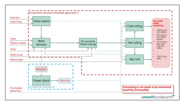
Figure 7-7 provides a complete monitoring approach for all source streams, for the example installation. In this figure a single bubbled system boundary has been drawn around production processes 1 to 4, for iron or steel products. Within the bubble, direct and indirect emissions for this production route result from:
