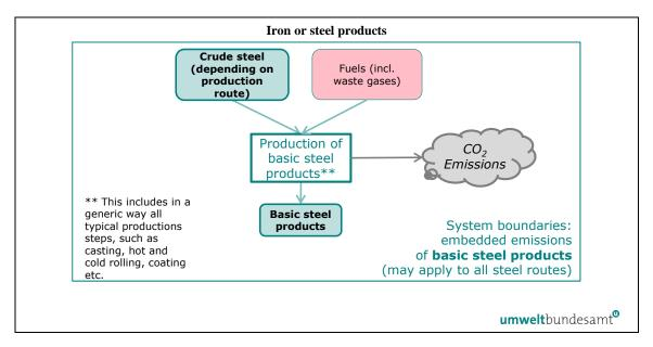
Figure 5-13: System boundaries of steel products production process
