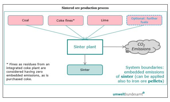
Figure 5-6: System boundaries of the sintered ore production process
