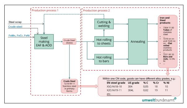
Figure 7-8: Example installation producing high-alloy steel from EAF route – Overview
