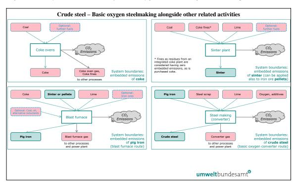
Figure 5-11: System boundaries of basic oxygen steelmaking and related processes.
